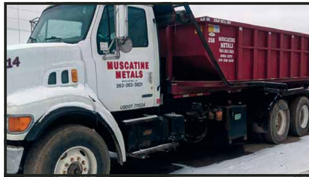
1999 Stirling Tandem Axle. Equipped with a Hesco T-1 roll-off body.
