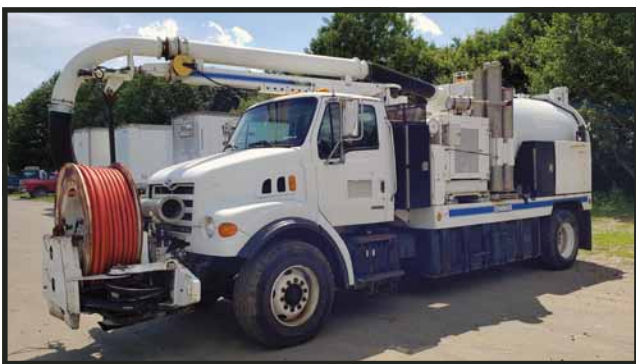
Vac-Con Vacuum Truck Sterling Chassis with Vac-Con body.
