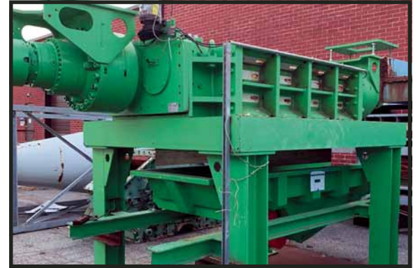
2016 ERDWISCH DUAL SHAFT SHREDDER 78" x 53" cutting chamber. (2) 120 HP motors.
