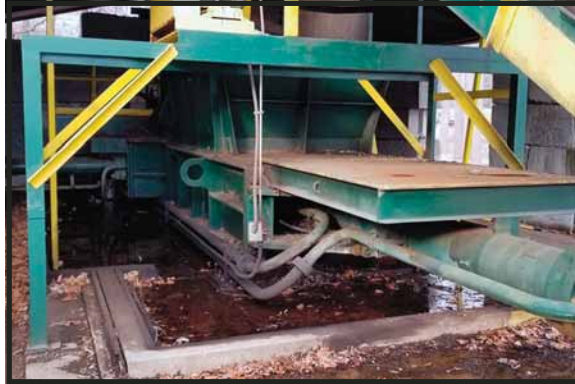
HARRIS HRB-NF TWO-RAM BALER Recent liners. USS auto-tie.
