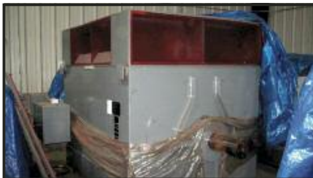
GE 3000HP Shredder Motor. In storage. 60Hz, 4,160 Volt, 712 RPM.
