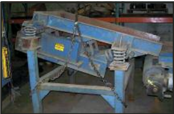
32" EDDY CURRENT SORT SYSTEM Includes 32" vibratory conveyor, control panel.
