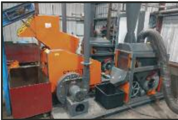
STRIP-TEC MODEL 600 WIRE GRANULATOR Includes a Worldwide pre-chopper.
