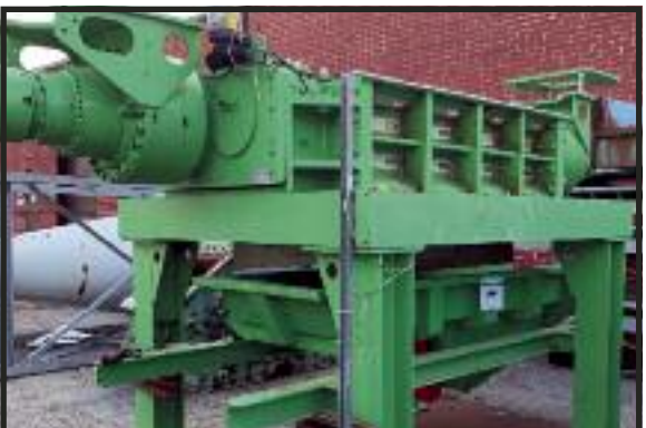
2016 ERDWISCH DUAL SHAFT SHREDDER 78" x 53" cutting chamber. (2) 120 HP motors.
