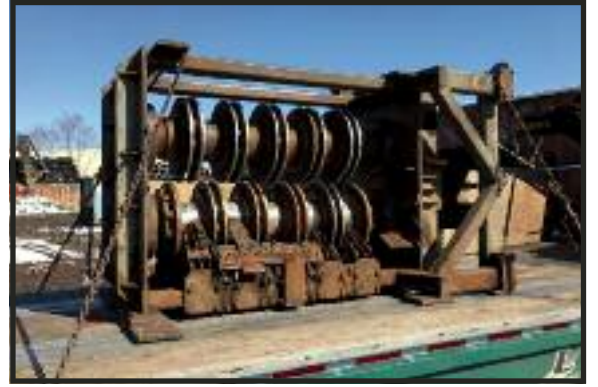
1999 BARCLAY ROTO-SHRED TIRE SHREDDER Bearings and frame are in good shape.
