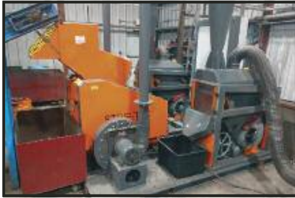
STRIP-TEC MODEL 600 WIRE GRANULATOR
