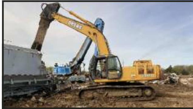
2005 John Deere 330LC. Equipped with a 2011 Genesis 440R shear.
