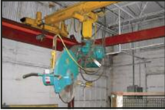
VULCAN FOX MODEL 2C-40 CUT-OFF SAW 40" blade. Includes overhead crane.
