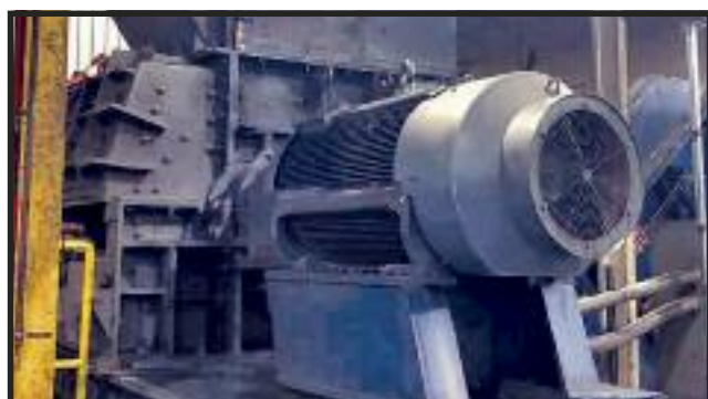
2014 American Pulverizer 48 x 50 Ring Mill Shredder. 500HP. New rotor recently installed! Infeed and outfeed conveyors.
