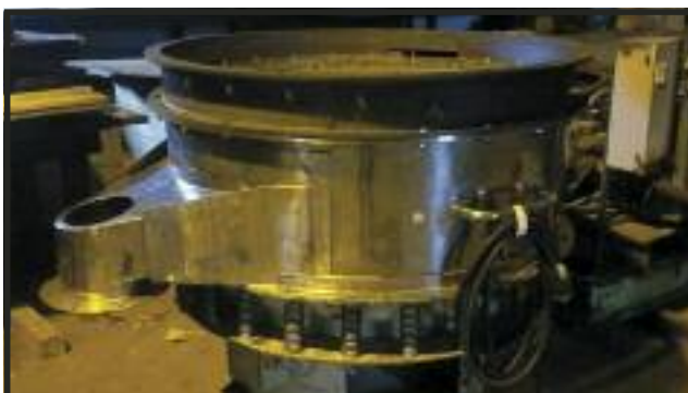
Sweco 48" Dual Deck Screener. Stainless steel decks and screens.
