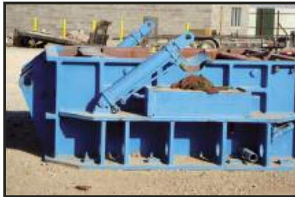
JEFFREY 60 x 90 HAMMERMILL SHREDDER Model 893. 800 HP motor.
