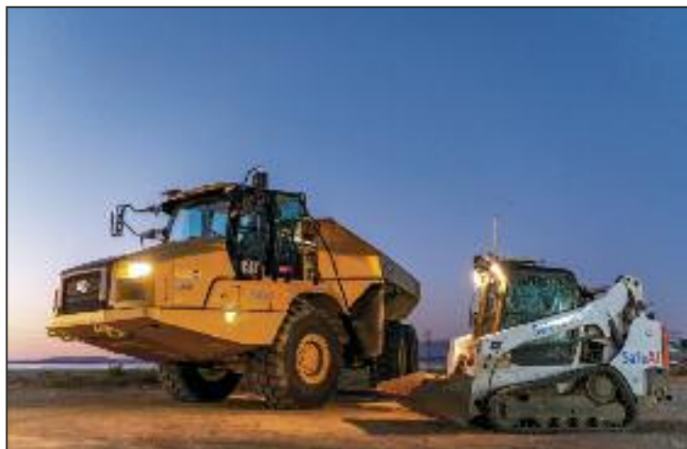
Goodyear recently retrofitted a Caterpillar 725 with autonomous software by SafeAI, keying in to the benefits of artificial intelligence for multiple industry segments.
