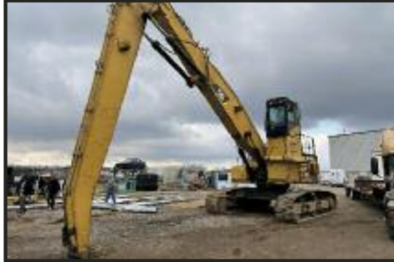
CATERPILLAR 345C MATERIAL HANDLER
