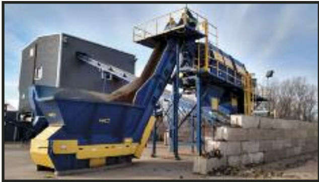
Complete Wendt Non-Ferrous Sort System.
