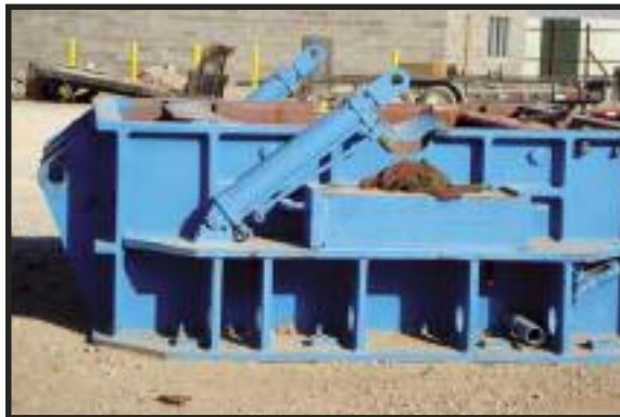
JEFFREY 60 x 90 HAMMERMILL SHREDDER Model 893. 800 HP motor.
