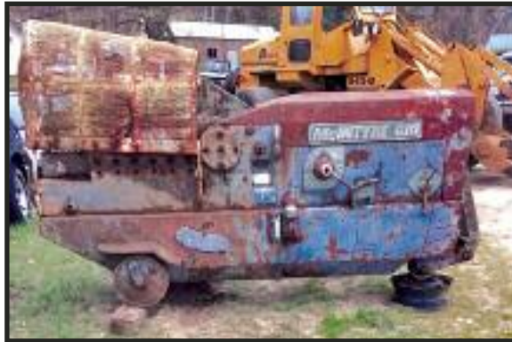
MCINTYRE 610 ALLIGATOR SHEAR 3 phase. 24 inch blade.
