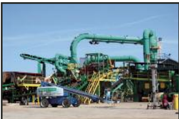
UNIVERSAL 74 x 104 HAMMERMILL SHREDDER 3500HP with ferrous line!
