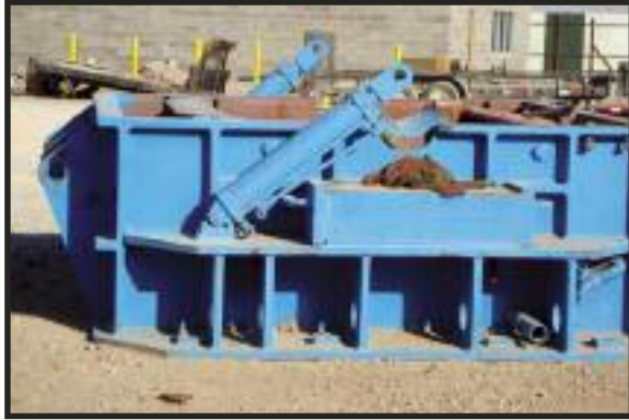
JEFFREY 60 x 90 HAMMERMILL SHREDDER Model 893. 800 HP motor.
