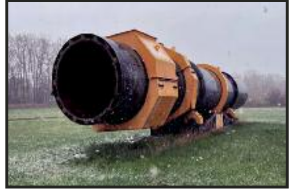
2005 DIDION ROTARY DRYER 96 inch diameter. 50 feet long.
