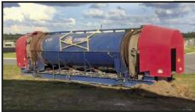
Dragon Dryer Rotating Biosolids Dryer. Indirect heat dryer. Previously used on rubber chips.
