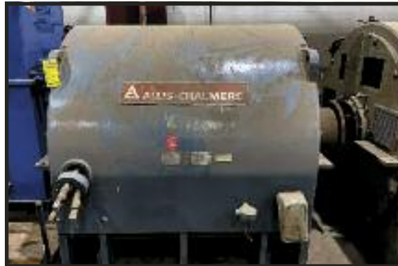
ALLIS CHALMERS 3,500HP MOTOR 698 RPM. 453 Amps. 3 Phase.
