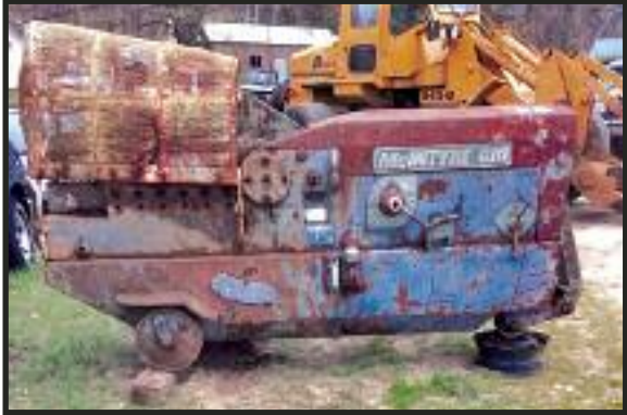
MCINTYRE 610 ALLIGATOR SHEAR 3 phase. 24 inch blade.
