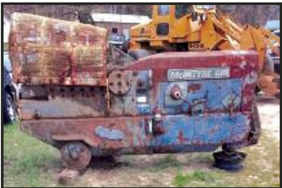
MCINTYRE 610 ALLIGATOR SHEAR 3 phase. 24 inch blade.
