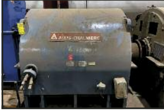
ALLIS CHALMERS 3,500HP MOTOR 698 RPM. 453 Amps. 3 Phase.
