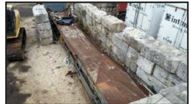
General Kinematics Vibratory Table. 45' long and 10' wide.
