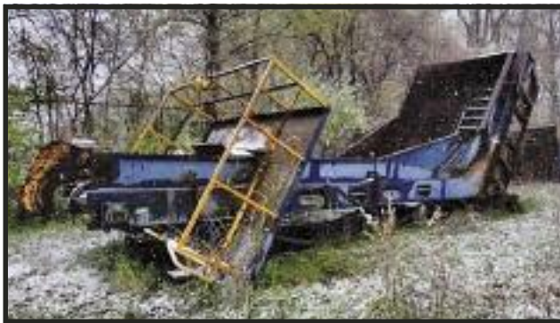
Wendt Tumble Back Feeder. 12' load area. 27' tall.
