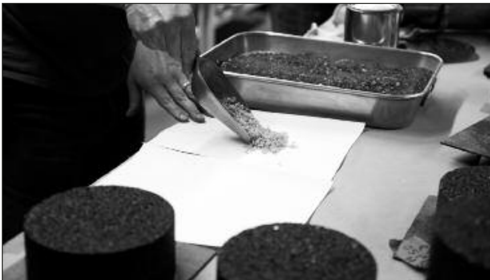
Lab staff in the Mizzou Asphalt Pavement and Innovation Lab, or MAPIL, show the plastic waste particles that are being added to the pavement mixture. The lab is located inside the MU College of Engineering.
