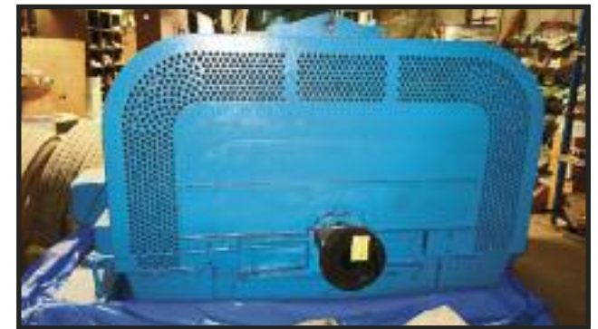
Allis-Chalmers 1,000HP Shredder Motor. 700 RPM 4,000 Volt
