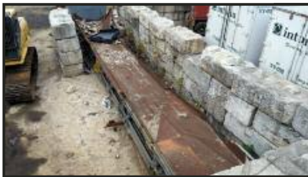
General Kinematics Vibratory Table. 45' long and 10' wide.
