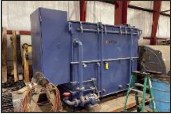
ELETELE 5000 HP LIQUID RHEOSTAT
