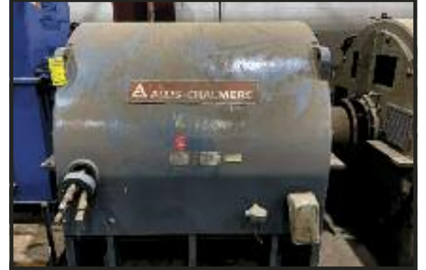
ALLIS CHALMERS 3,500HP MOTOR 698 RPM. 453 Amps. 3 Phase.
