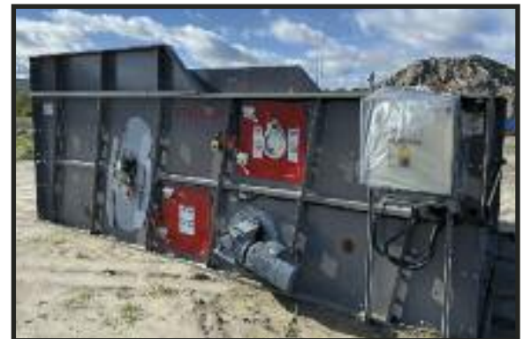
STADLER BALLISTIC SEPARATOR STT-2000-8
