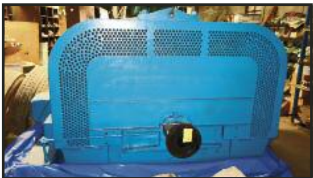
Allis-Chalmers 1,000HP Shredder Motor. 700 RPM 4,000 Volt
