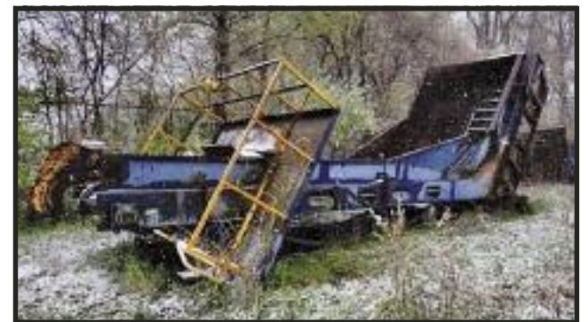
Wendt Tumble Back Feeder. 12' load area. 27' tall.
