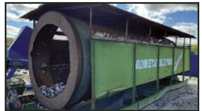
Tuffman Model 722 Trommel. 7' wide by 22' long
