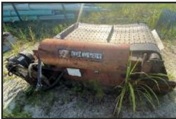
ERIEZ MAGNETICS OVERHEAD MAGNET 36" x 6'. Dual Pole Rotor.
