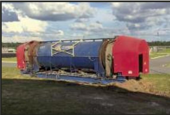
DRAGON DRYER INDIRECT ROTATING DRYER Two indirect dryers. Use with ASR or biosolids.
