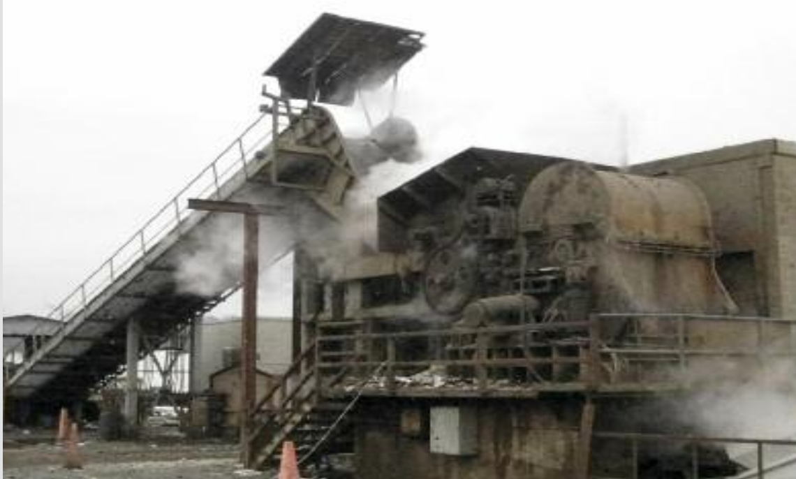
Innovative Shredder System 60x66, Infeed Conveyor Flat Loading Section, Infeed Conveyory Incline Section, Infeed Ramp, Double Feed Roll Assembly, Shredder Lower Box Section, Shredder Rotor
