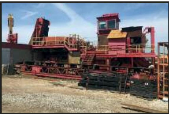
SMC 1000 TON PLATE SHEAR Used to cut railroad car sides and other plate.
