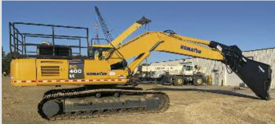
PC-400 DASH 6 Genesis GXP 990R Genesis Shear 100% Rebuild with Jaw Armor Installed PC-400 Totally Gone Through
