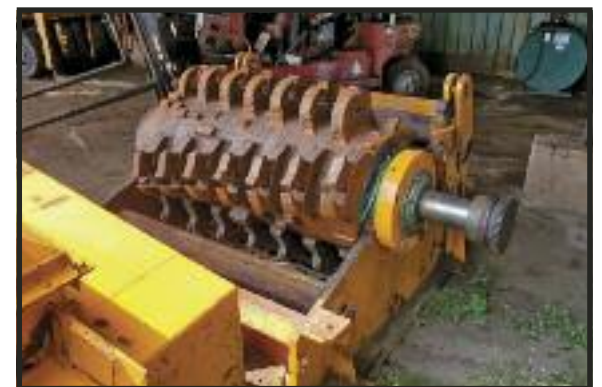
CBI GRIZZLEY MILL 4872 Used for wood and e-waste.
