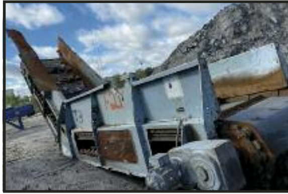
RUBBER-OVER-CHAIN INFED CONVEYOR 60" wide by 25' long.
