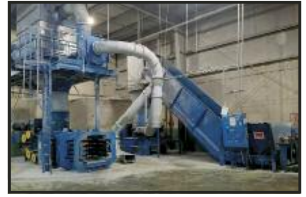
BALEMASTER CONTINUOUS BALER Automatic baler with electric bale tier.
