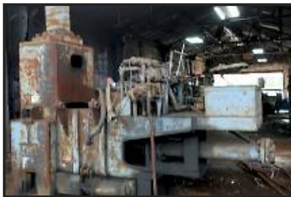
HARRIS NF50 BRIQUETTER Three-ram non-ferrous briquetter.
