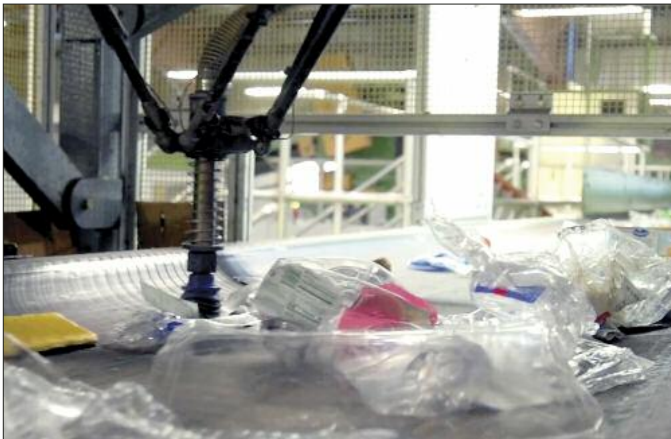
An AMP robot, guided by artificial intelligence, sorts material on a container line.
