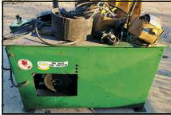
IFM 2000 TIRE STRIPPER Model 818. Used on forklift tires.
