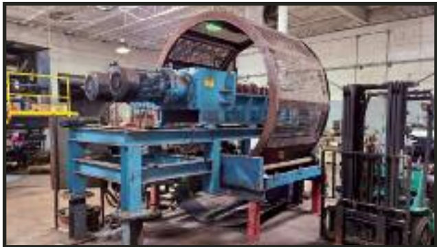
ShredPax AZ80 Hook Shear Shredder. Includes trommel assembly and hopper.
