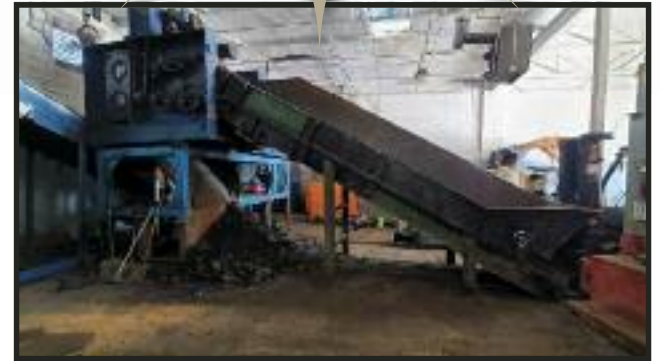
1995 AmeriShred Tire Shredder. 4.5" cut. Includes conveyance.
