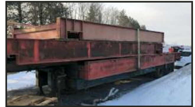
Thurman 70' Truck Scale. 200,000lb capacity. Concrete deck.
