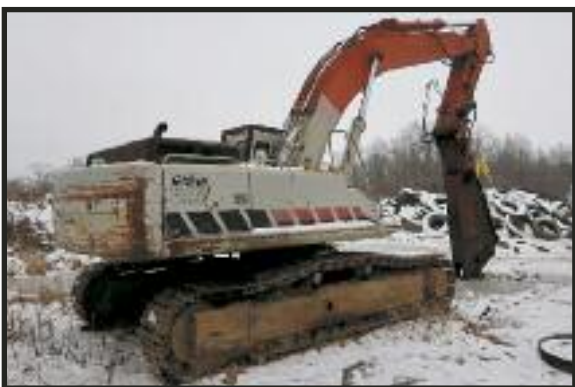
LINK BELT EXCAVATOR WITH LABOUNTY SHEAR
