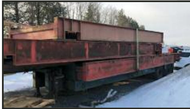
Thurman 70' Truck Scale. 200,000lb capacity. Concrete deck.
