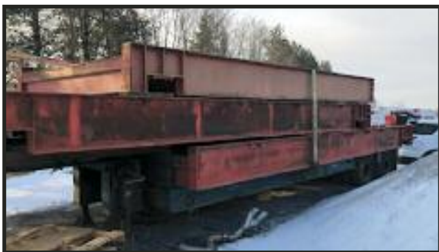
Thurman 70' Truck Scale. 200,000lb capacity. Concrete deck.
