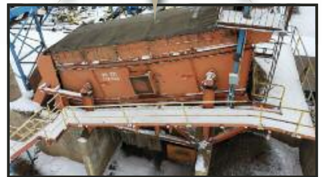
Bivi Tech KRL DD 3000 X8. Processes 50-55 TPH of ASR.
