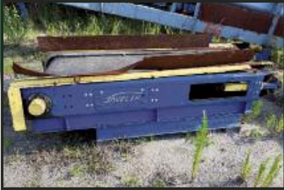
JAVELIN EDDY CURRENT SEPARATOR 36" wide by 12' long.
