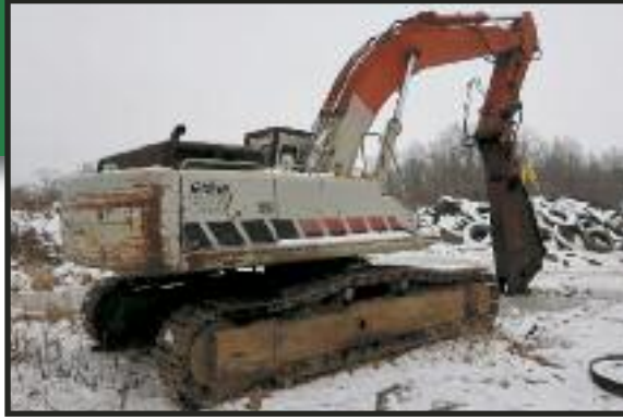
LINK BELT EXCAVATOR WITH LABOUNTY SHEAR
