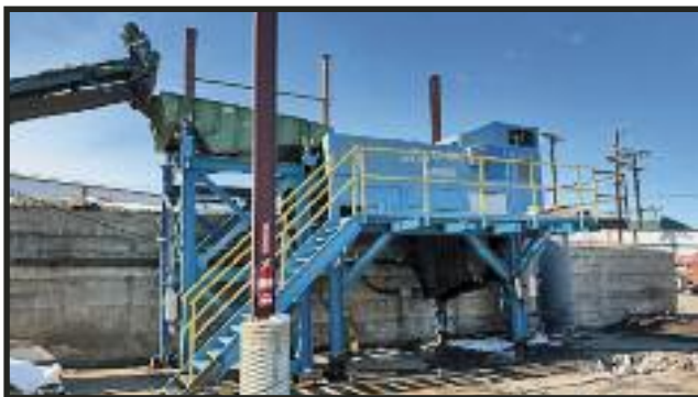
2013 SGM Sensor Sort and Peripherals. Model EMS-EF-R96. Includes feeder.
