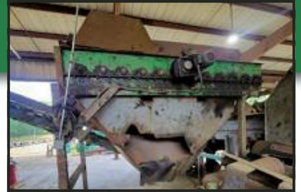
JOMAR DAISY WHEEL CLASSIFIER Set up for 3" cut.
