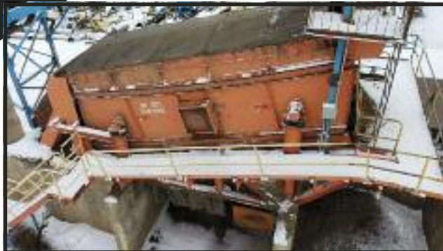
Bivi Tech KRL DD 3000 X8. Processes 50-55 TPH of ASR.
