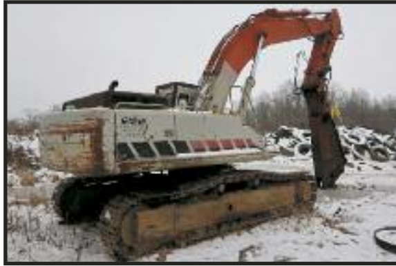
LINK BELT EXCAVATOR WITH LABOUNTY SHEAR
