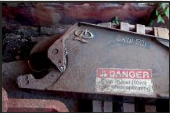
LABOUNTY MSD 7R SHEAR Was used on a Bobcat. Jaw opens 10".
