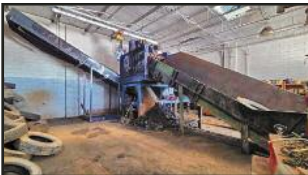
1995 AmeriShred Tire Shredder. Produces a 4.5" cut. Will shred truck tires.
