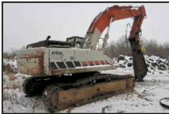
LINK BELT EXCAVATOR WITH LABOUNTY SHEAR
