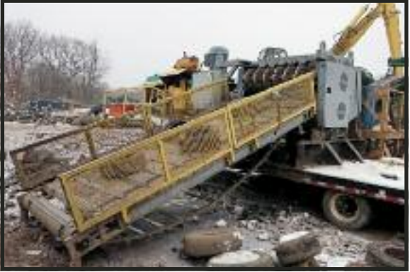
BARCLAY PORTABLE TIRE SHREDDING LINE
