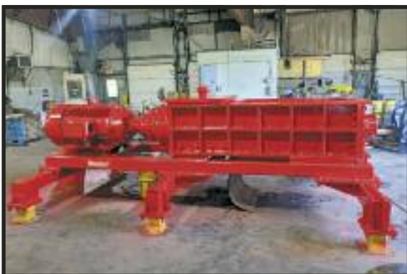
R-TECH HD 3850 DUAL SHAFT SHREDDER 250HP. 50" x 38" FEED OPENING.
