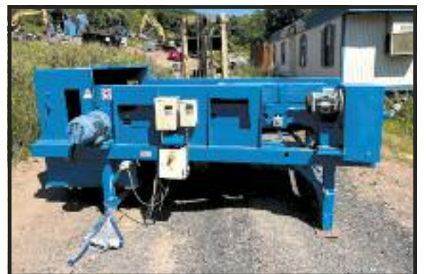
2006 SGM VIS 60 EDDY CURRENT 60" BELT WITH VIBRATORY FEEDER.
