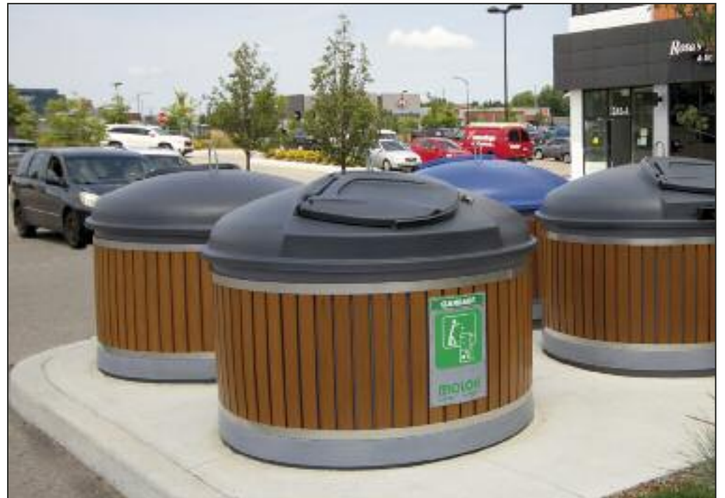
Molok creates waste containers that utilize the coolness of the ground to minimize odors. The oldest waste is at the bottom, in the coolest part of the container and utilizes gravity for compaction using its own weight. This allows each container to hold approximately 20 percent more waste. PHOTO COURTESY OF MOLOK LTD.
