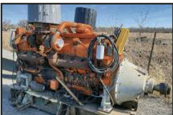
DETROIT DIESEL ENGINE WITH SHIV SYSTEM 1,515HP. TWIN DISC CLUTCH.
