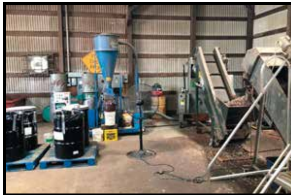
CABLE MANAGEMENT WIRE CHOPPING SYSTEM INCLUDES CABLE SHREDDER AND GRANULATOR.
