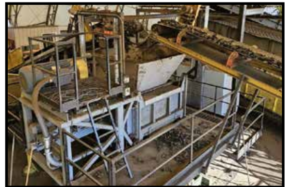
2" BARCLAY / CM TDF SHREDDING SYSTEM BARCLAY 2" AND CM 1.7" TDF TIRE SHRED LINE
