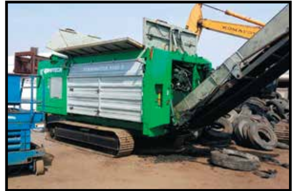
KOMPTECH TERMINATOR 5000 SD THIS TRACKED SHREDDER IS READY TO WORK!
