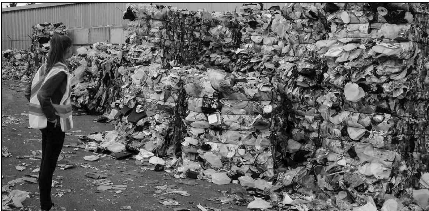
Plastics are sent to material recovery facilities (MRFs) where they are sorted and baled.
