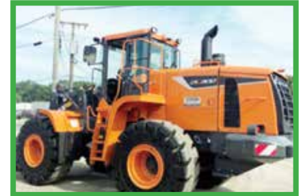
2018 Doosan DL300-5K-US11 S/N: 076, Hydraulic Locking Front Differential, Quick Coupler, 4.5 Yard Bucket $135,000
