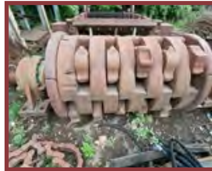
SHREDDER ROTOR In good shape | Bearings and housings mounted on the rotor | Recappable end discs | Motor drive coupling mounted on the shaft | Full set of hammers and pin protectors mounted on the rotor
