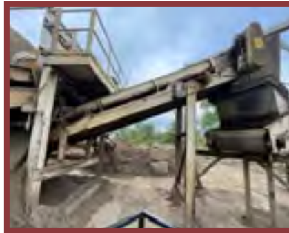
C3 NON-FERROUS CONVEYOR Length 20 feet | Width 36 inches HP 7 1/2 | Speed 175 FPM
