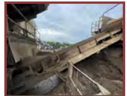
C1 PRIMARY FERROUS CONVEYOR Length 25 feet Width 54 inches HP 7 1/2 Belt speed 175 FPM Picking Station
