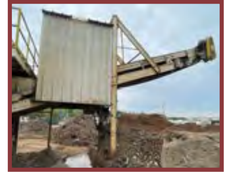
C2 FERROUS STACKING CONVEYOR Length 28 feet Width 48 inches HP 7 1/2 Belt Speed 175 FPM
