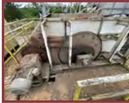
MAGNET STAND 48" x 60" Permanent Magnet With drum drive chain driven With lower fluff chute Catwalk on drive side of the drum
