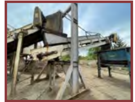
C4 2nd NON-FERROUS CONVEYOR Length 20 feet Width 36 inches HP 7 1/2 Speed 175 FPM
