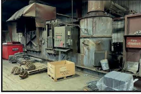
AL-JON / UNITED F466 EW SMELTING FURNACE 1,000-1,200 LBS/HR OF MELT. 4,000LB HOLDING CHAMBER. 5 SOWS.
