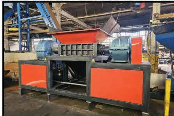
NEW DUAL SHAFT HOOK SHEAR SHREDDER 150HP. HIGH TOOTH COUNT BLADES. GREAT FOR TURNINGS!
