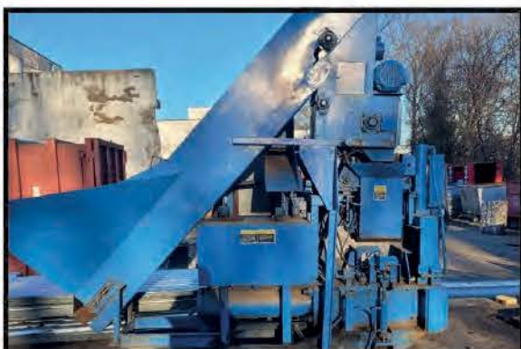
MOSLEY ALUMINUM CAN DENSIFIER INCLUDES INFEEED WITH HOPPER AND CONTROLLER. 3 PHASE.
