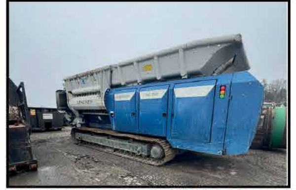
2020 LINDNER URRACO 95 DK MOBILE SHREDDER TWIN SHAFT, LOW RPM, MOBILE SHREDDER. 750HP.
