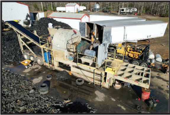
JORDAN MS5040 PORTABLE TIRE SHREDDER (2) 200HP MOTORS. SHREDS TIRES ALL DAY LONG!
