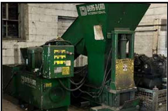
2008 DENS-A-CAN 1200 CAN DENSIFIER 11 X 13 X 9 BALE SIZE. CAN HANDLE UBC AND STEEL CANS.
