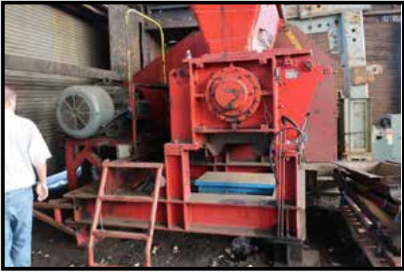
CIMP RUBBER GRANULATOR LINES TWO LINES. EACH LINE INCLUDES 2 GRANULATORS AND CONVEYANCE
