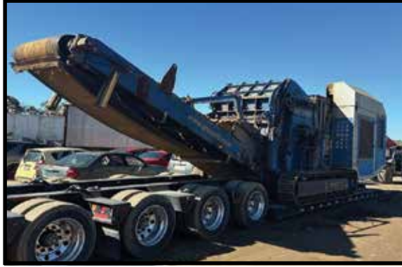
ZB THOR 1616K TRACKED HAMMERMILL DENSIFIER 755HP CAT DIESEL ENGINE. 2018 MODEL YEAR.
