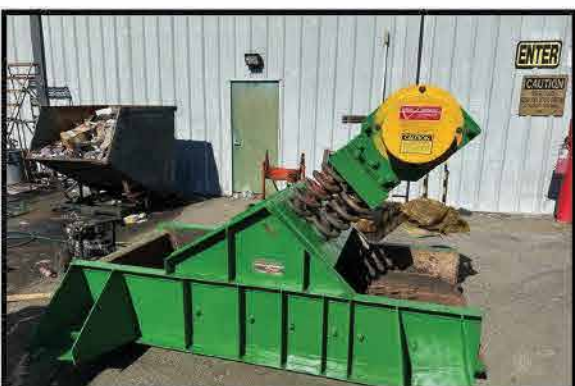
36" X 8' PARA-MOUNT II VIBRATORY FEEDER COMBINATION VIBRATORY FEEDER AND FINGER SCREEN
